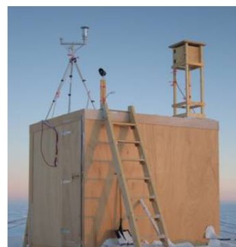
Fig. 1 - Shelter for aerosol sampling
